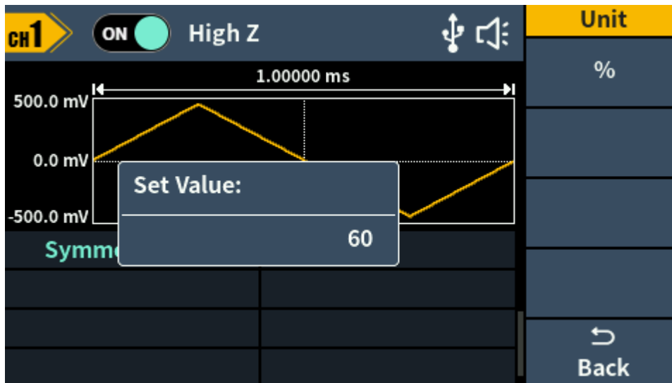
Figure 5-6: Set the symmetry of ramp wave
