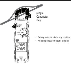
$\bullet$  AC Amps can be measured in any position of the rotary selector dial.
