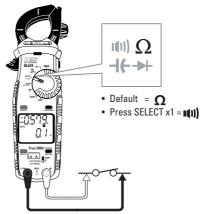
• Buzzer sounds at less than  $< 40\Omega$ .
