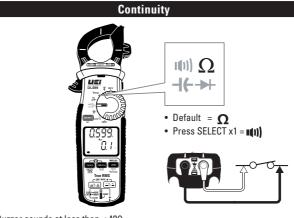
• Buzzer sounds at less than <  $40\Omega$ .
