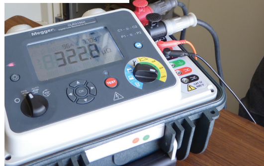
DLRO100H testing rack-mounted, 3-phase circuit breakers
