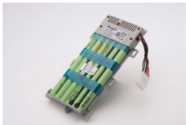
A user replaceable high power lightweight Li-ion battery provides, from a single charge, 200 Manual/Auto 100 A tests or up to two 10 minutes continuous 100 A tests and takes 2.5 hours to charge when fully discharged.
