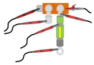
This is an example of how the Kelvin probes or Kelvin clips can be used. In this case a clip is attached to the bus bar and a probe is used to quickly and accurately measure each point of connection.
