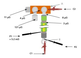
**Note:** Cable length A to B >5 m, resistance >2.5 m $\Omega$  (approx)
