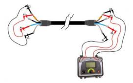
Take the instrument to the working end of the long cable and connect to the two cores selected to be the P1 and C1 connections. Connect the P2 and C2 test leads to the core to be measured as shown.
