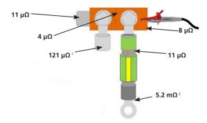
As seen in this example, a DLRO or Ducter provides accurate results. By comparing similar connections a number of potential hazards can be easily revealed:
