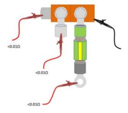
Due to the convenience, a multimeter or continuity tester will often be used to verify connections on industrial ground or power systems. These instruments are not designed for such applications and cannot measure extremely low resistance to highlight the small increases that will waste energy or even render ground systems much less effective.
