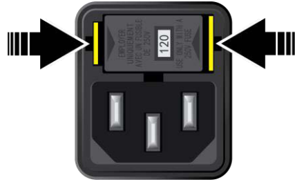
Figure 146: DMM6500 AC receptacle and line fuse location
