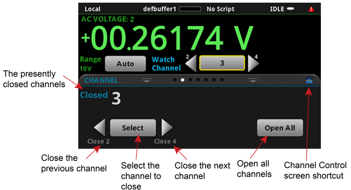
Figure 44: Channel swipe screen
