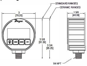
The **SERIES DPG-000** Digital Pressure Gage has a precise  $\pm 0.50\%$  full scale accuracy. The 4 digit digital display will reduce the potential for errors in readings by eliminating parallax error commonly produced with analog gages.
