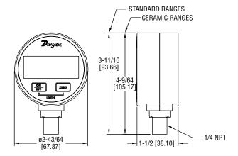
The **SERIES DPGA & DPGW** Digital Pressure Gages have a precise ±1.0% full scale accuracy. The 4 digit digital display will reduce the potential for errors in readings by eliminating parallax error commonly produced with analog gages.
