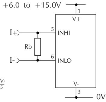
Measuring a current from a circuit which is floating with respect to the DPM's supply, i.e. the current and the meter's power supply are isolated from each other.
