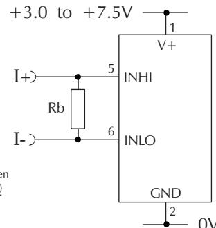
Measuring a current from a circuit which is floating with respect to the DPM's supply, i.e. the current and the meter's power supply are isolated from each other.
