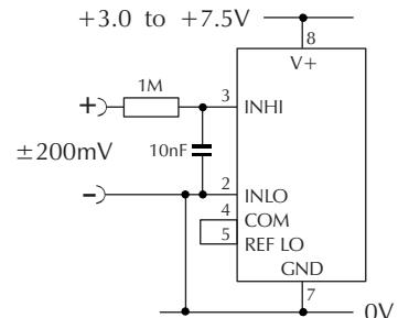
Measuring a single ended input voltage referenced to supply, i.e. the input voltage and the meter's power supply share the same 0V rail.
