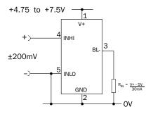
Measuring a single ended input voltage referenced to supply, i.e. the input voltage and the meter's power supply share the same OV rail. Ensure solder link LCOM is open.
