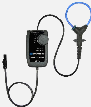
DRANFLEX300MHB 3A/30A/300A Probe Available in 6", 8" and 12"
