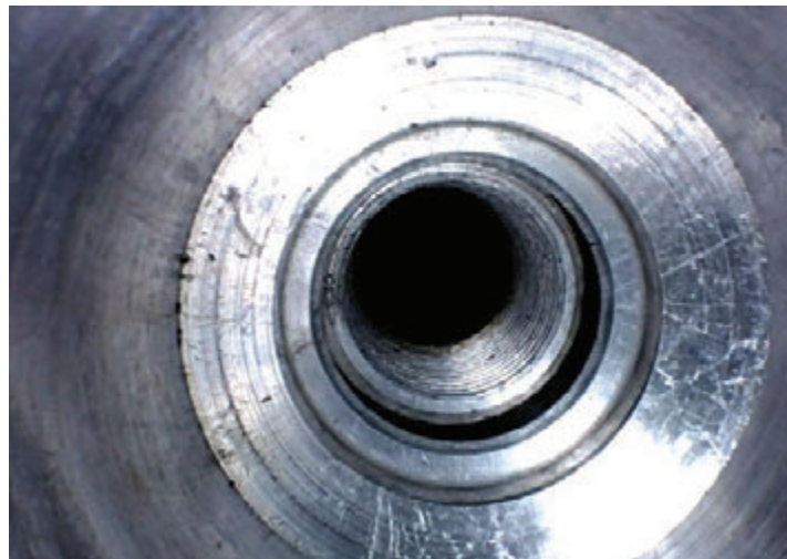
Photo above: Spark plug port inspection
