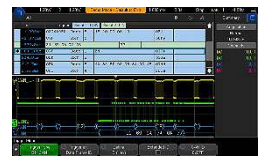
Figure 19. Multi-bus time aligned decode.
