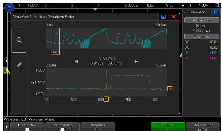
Figure 25. Optional arbitrary waveform generator provides easy access to stimulus. The integrated arbitrary waveform generator makes capturing, modifying and replaying signals simple.
