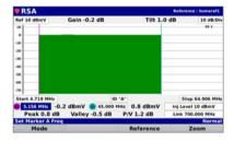
the 1G DSP to track up to 643 individual sweep points and display a full sweep on the screen every four seconds
