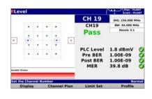
Provides Pass/Fail results for PLC Level, Pre-BER, Post-BER, and MER measurements when compared against user-defined limit sets
