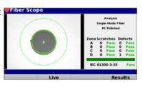
• Intelligent fiber microscope eliminates fiber inspection guesswork
