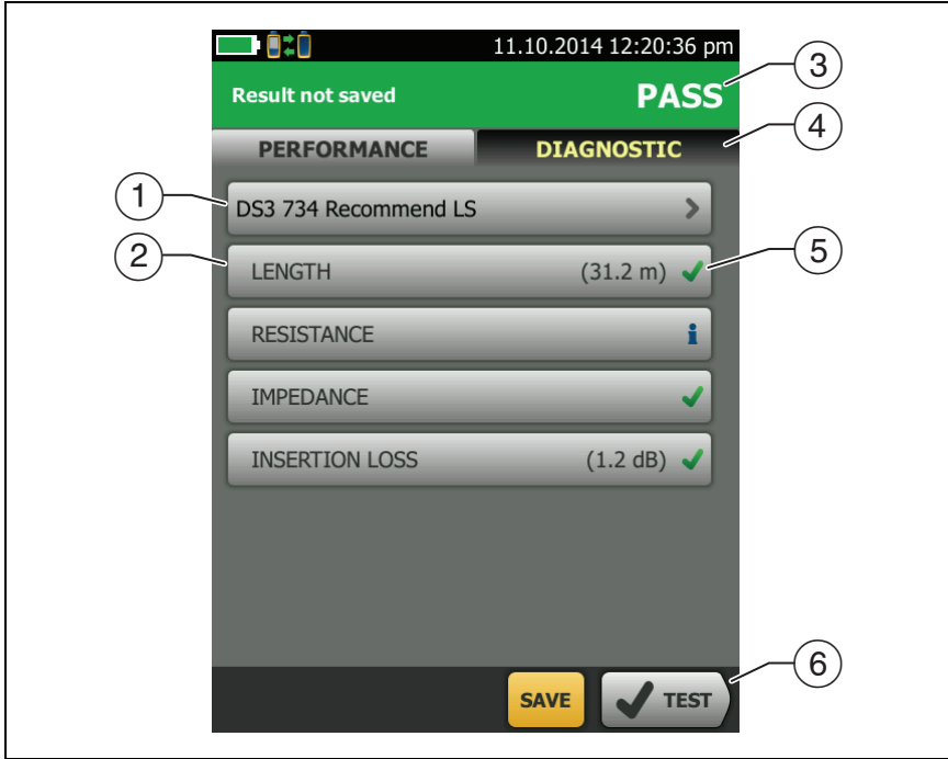
Figure 25. Autotest Results for Coaxial Cabling
