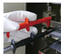
For clamping around the target busbar
