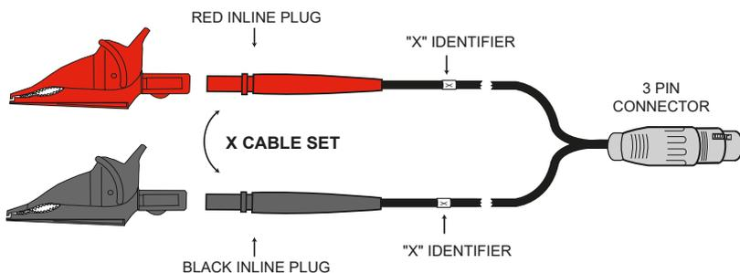
Each cable is clearly marked. The Primary (H) cable has a 5-pin connector and the Secondary (X) cable has a 3-pin connector. They cannot inadvertently be connected incorrectly.
