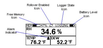
This screen shown the current Relative Humidity, Temperature and Dew Point measurements. The measurements
