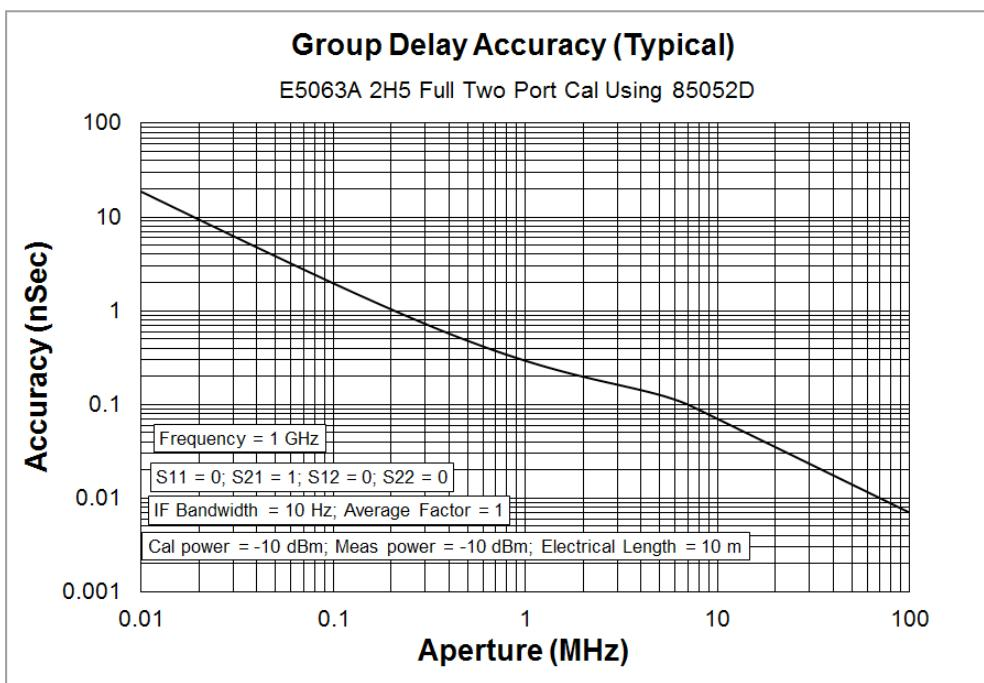
In general, the following formula can be used to determine the accuracy, in seconds, of a specific group delay measurement:
