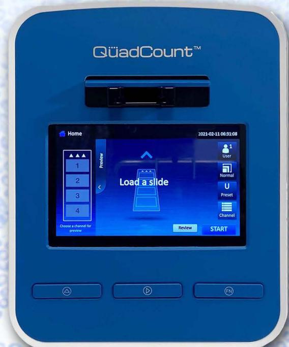
Correct focus is crucial for accurate counts of viable cells. The QuadCount's proprietary autofocus system and image analysis software work in conjunction with the motorized stage to analyze and capture images in the proper focal plane.
