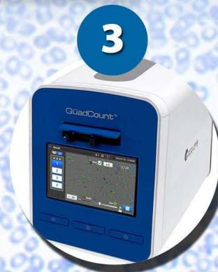
3 Insert slide into QuadCount™ and press START
