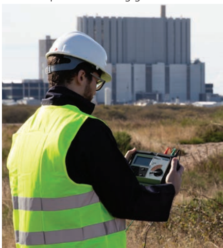
Typical use of a Megger digital ground resistance tester - the DET4TC - to perform fall-of-potential testing.
