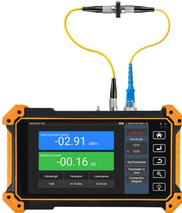
After setting the reference value, connect the optical device to the OTDR and LS interfaces on the instrument to test the insertion loss of optical passive devices. Click "Loss Test" under optical fiber tests to enter the interface.
