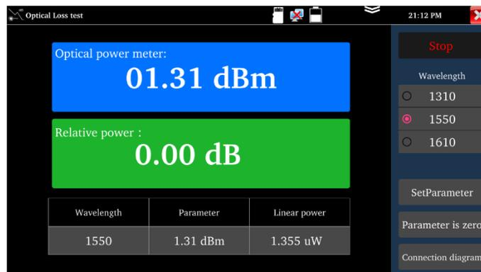
After setting the reference, connect the tested optical device to the meter's OTDR and LS ports and click "Start." The relative power displayed on the interface will be the insertion loss value of the tested device.
