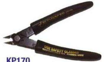
KP170 Micro-Shear Flush Cutter with Static-Safe Cushioned Grips and Non-Reflective Cutting Head. Flush Cuts Soft Copper Wire up to 20 AWG. L: 5.1" (130mm)
