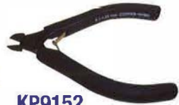
KP9152 Flush Cutter with Oval Head for Copper Wire: .004" (.1mm) - .049" L: 4.3" (110 mm)
