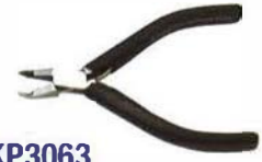
KP3063 Regular Bevel Oblique End Cutter Oblique Angle 11° for Copper Wire: .01in (.35mm)- .049in (1.25mm) L: 4.1" (105 mm)
