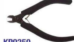
KP9350 Regular Bevel Cutter with Oval Head for Copper Wire: .012" (.3mm) - .063" (1.6 mm) L: 4.4" (112 mm)
