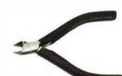
KP3056 Flush Cutter with Pointed and Relieved Jaws for Copper Wire: .001in (.35mm) - .039in (1 mm) L: 4.2" (107 mm)
