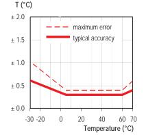
**SENSOR ACCURACY & INFORMATION** Typical and maximal tolerance for temperature sensor in °C.
