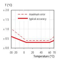
**SENSOR ACCURACY & INFORMATION** Typical and maximal tolerance for temperature sensor in °C.
