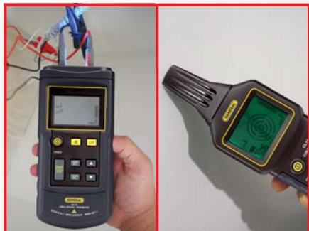
Tracing a cable behind a wall
