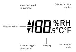
The LCD shows six different recorded readings, which can be cycled through using the built-in push button. The most recent logged value, maximum logged value and minimum logged value can be displayed separately for humidity and temperature. In addition, logging and alarm status is shown using two high intensity LEDs.
