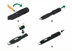
Before using the data logger you will need to insert the 3.6V 2/3AA High Temperature battery provided, following the instructions below.
