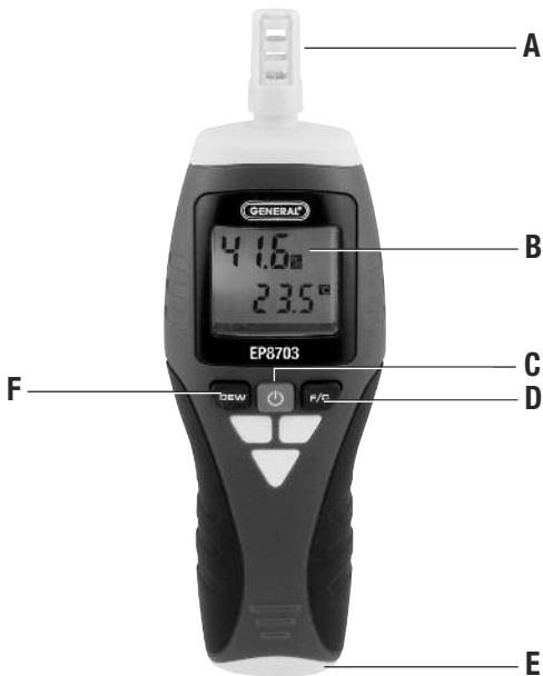
Fig. 1. The EP8703's controls, indicators and physical structures
