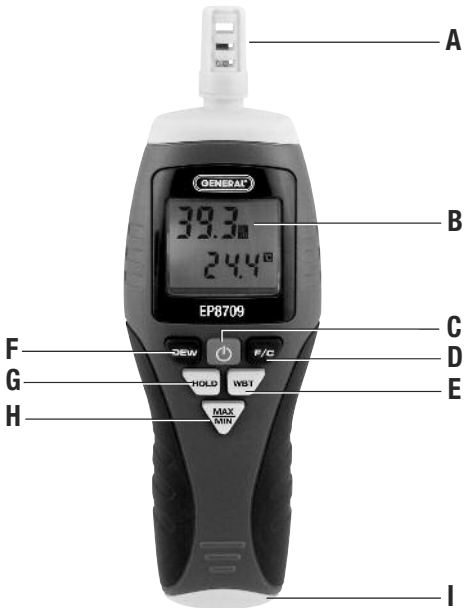
Fig. 1. The EP8709's controls, indicators and physical structures
