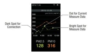
In the measurement page a LONG PRESS of the MEM/Down button enters and exits the memory page.
