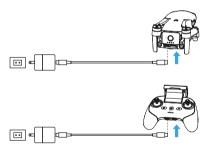
Fully charge the aircraft batteries and remote control before flying.
