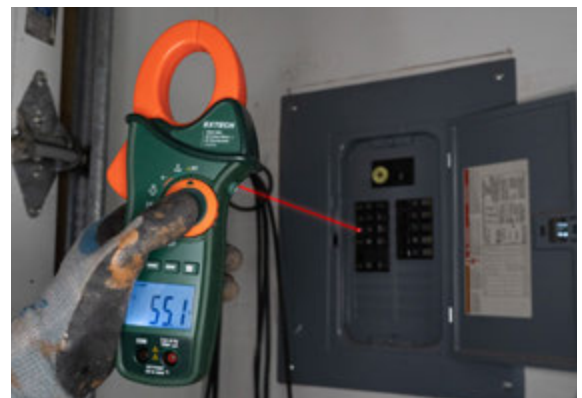
Built-in IR thermometer with laser pointer for locating hot spots and overheating motors.
