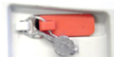
Locked with Wire Seal
