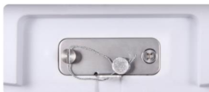
Locked with Wire Seal
