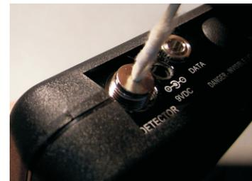
5 Using as little pressure as possible, rotate the cotton toothpick tip in the detector port to clear away any dust or dirt that has accumulated on the detector.
