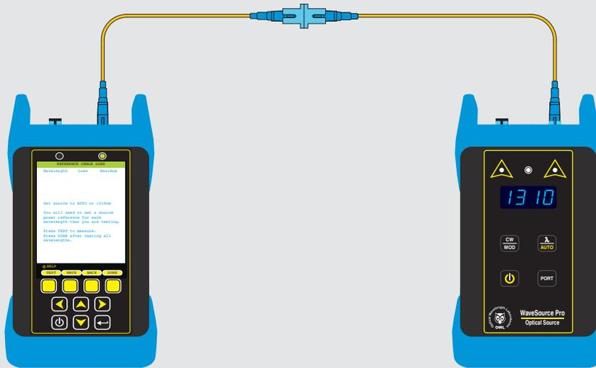
**17** After a few seconds, the **REFERENCE CABLE LOSS** will be shown. (NOTE: If Loss exceeds Maximum, it is recommended to replace the additional test cable and/or mating sleeve.) Press **DONE** to record the **REFERENCE CABLE LOSS** and continue.
