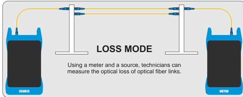
**Optical Power Measurements.** Optical power is an absolute measurement of the amount of light intensity; i.e. "brightness", and can be measured either at the output of a transmitter (transmit power), or at the input of a receiver (receiver sensitivity). When in OPM mode, Fiber OWL 7 certifiers can be directly attached to this equipment via a patch cord to check whether the transmitter is within the manufacturer's specified power range.
