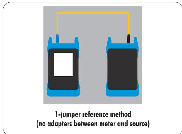
For non-standard link configurations, such as a patch panel on one end, or “home run” (i.e. no patch panels), technicians may need to adjust their test procedure and reference method accordingly.
