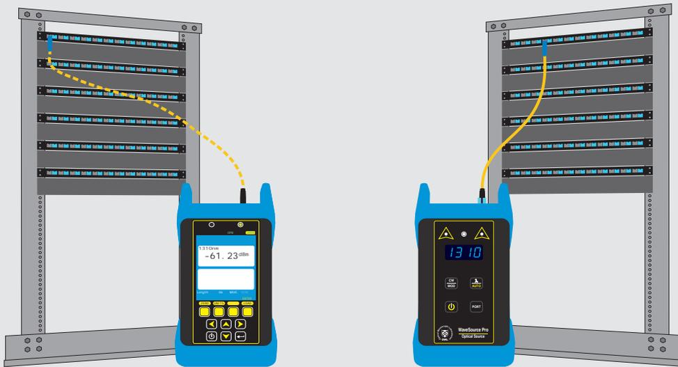
**Once the meter is connected to the same fiber (continuity achieved), a reading that is close to the light source's calibration power level will appear.**
