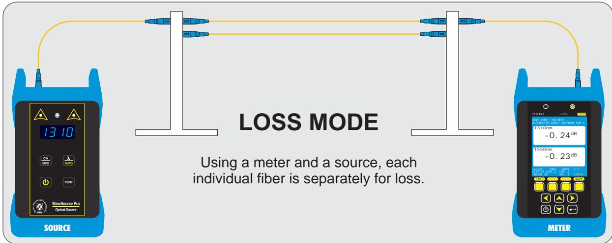
LOSS MODE can be performed with all models of **FIBER OWL 7 optical power meter** and standalone light source (purchased separately or as part of a certification test kit).
