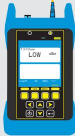
Press WAVE until the meter is set to the same wavelength as the network equipment. Press UNITS until the meter is set to display optical power in dBm.
