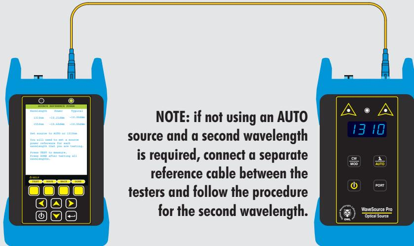
**NOTE:** if not using an AUTO source and a second wavelength is required, connect a separate reference cable between the testers and follow the procedure for the second wavelength.
