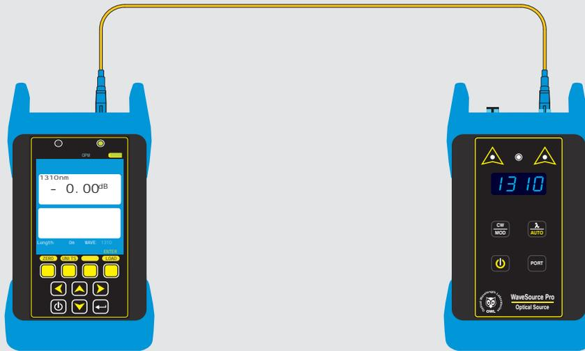
**Connect the METER and source into the first fiber in the link under test as shown. The meter will begin to display loss readings automatically.**
