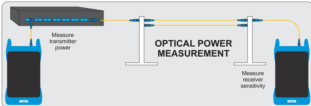
**Fiber Continuity Testing.** Continuity can be measured with OPM mode in the Fiber OWL 7 by placing a calibrated light source on one end of the fiber and the meter on the other end. This is also a simple way to measure the attenuation of the fiber.
