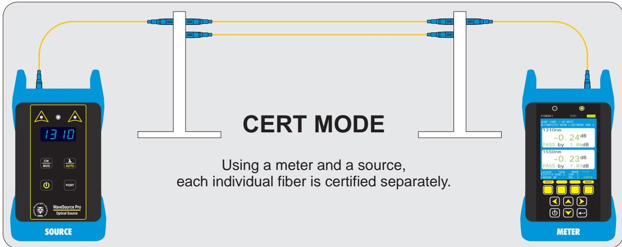
CERT MODE can be performed with all models of **FIBER OWL 7 optical power meter** and standalone light source (purchased separately or as part of a certification test kit).
