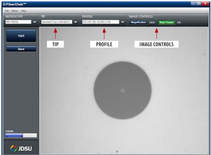
**MICROSCOPE** Allows the user to select the specific microscope they want to have active for displaying on the screen. If multiple microscopes are connected, each one will appear in a drop down list.
