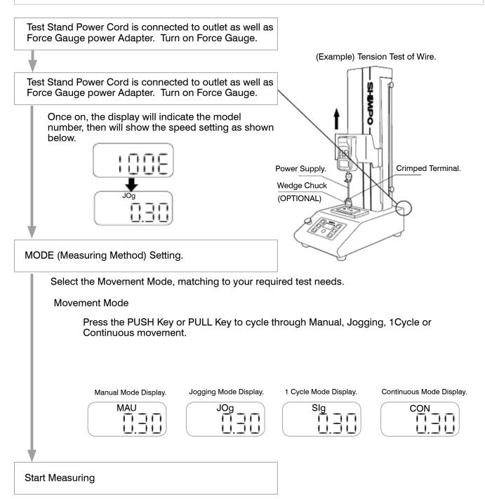
With the PUSH or PULL Key, Measurement can be started. For details refer to the Movement Mode Operation described later. Load Tests as follows can be performed.
