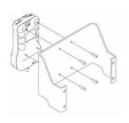
Using the Allen wrench spanner provided in the accessories, remove the installation bolts connecting the Test Stand and the Force Gauge Mounting Bracket
