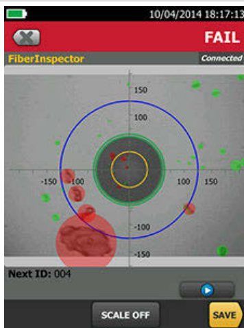
Defects that fail the standard's requirements are colored Red
