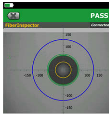
Defects that pass the standard's requirements are colored Green
