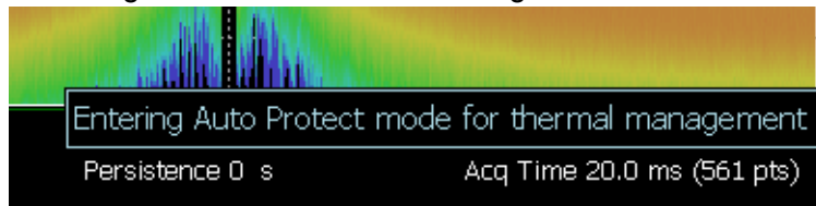
Figure 2-1 Entering Auto Protect mode message (above ~64°C)—(Displays for 3 sec)
