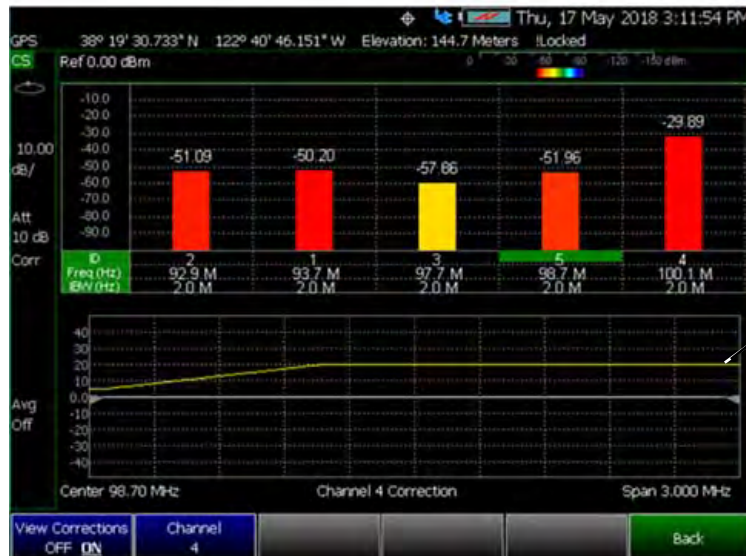
Figure 23-16 Yellow Trace with Cable and Antenna Corrections
