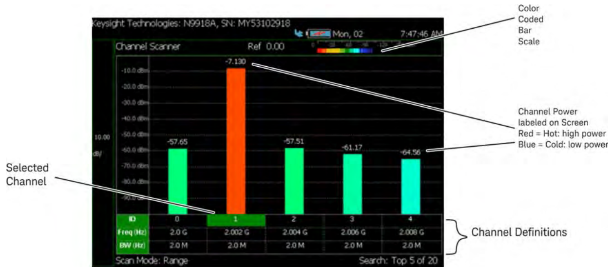
Figure 23-1 Display Example: Measure 5 Channels Spaced 2 MHz Apart
