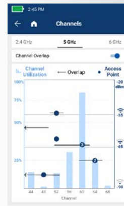
Channel test shows key information for understanding the Wi-Fi environment: number of AP's seen on and overlapping each channel and their signal strength, plus total channel utilization. Touching a channel provides details on APs on or interfering with that channel.
