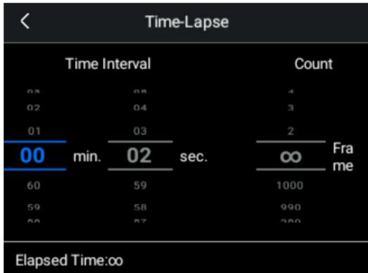
1. Users can set intervals between taken photos, shortest being 2 seconds and longest being 60 minutes 59 seconds.
