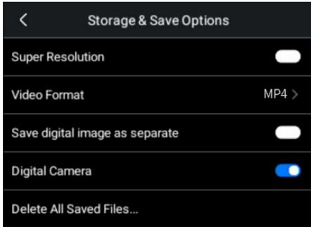
1. Super resolution: when turned on, the digital resolution of thermal images will double. This function is not available under video recording and time-lapse mode.
