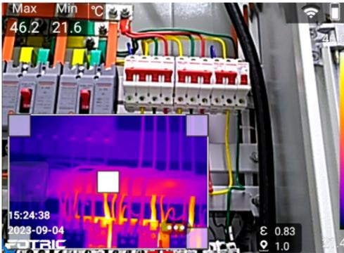
3. When specific ROI is selected, 'Resize' and 'reposition' mode can alternate by pressing the 'OK' button. Pressing the 'Return' button can exit editing mode.
