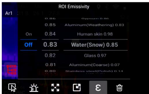
For the emissivity of material that is not included in the chart, you may find it in the emissivity table at the end of this manual.
