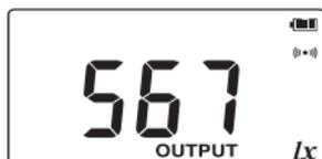
The voltage is output from the D/A OUTPUT terminal, depending on the measured value. ( **OUTPUT** appears.)
