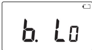
When the charge is gone, **[b. Lo]** flashes on the display for 3 seconds and the power is shut down automatically.
