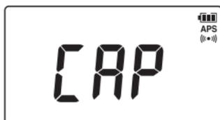
If you press **0ADJ** without the included sensor cap attached to the illuminance sensor (when the count is equivalent to 1 lx or greater), **[CAP]** will be displayed on the LCD.
