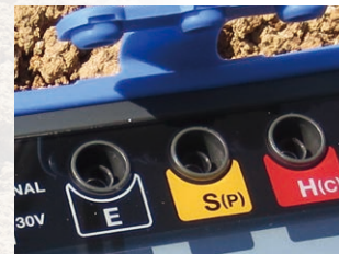
IP67 protection, even with the terminal caps open
