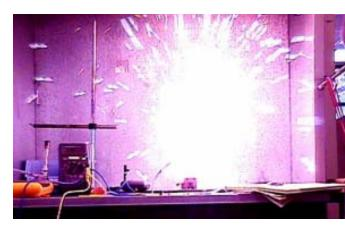
the high temperatures (up to 10,000 °F) generated by the energy will melt the sand and turn it to glass. The glass coats the element and smoothers the fireball by cutting off the available oxygen, keeping you and the tester safe from harm.
