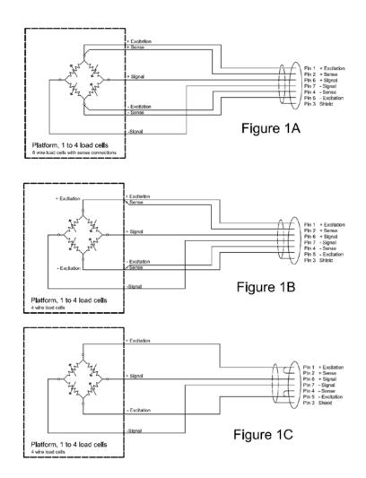
Figure 1A shows the connections to a 6 wire load cell. Figure 1B and 1C show 2 different ways to attach a 4 wire load cell, 1B uses a 6 conductor cable to go from the indicator to the platform or load cell where it connects to the 4 wires from the load cells.
