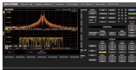
GDS 3000A has a built in Web Server function to allow users to connect GDS 3000A's Web Server by using a browser in the same network domain via Ethernet connection. System information can be obtained and the oscilloscope screen (. png file) can be observed and captured remotely.
