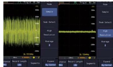
The acquisition method with high resolution mode is provided to effectively remove noise and improve the accuracy of automatic measurement.
