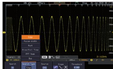
Users can rapidly search desired waveforms according to the trigger condition. After activating the search function, hollow inverted triangles will show the location met the trigger condition. The upper left hand corner Overall will show the total number of waveforms met the trigger condition. Users can set waveform search by the trigger condition such as Edge, pulse width, Runt, Rise/Fall, and Bus.
