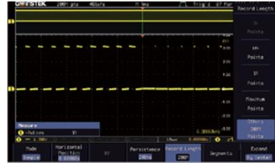
The GDS 3000A series oscilloscope has a powerful and incomparable memory depth for the data retrieving. 200M memory depth per channel independently surpasses the specification of the industry's 3000 series DSO boundary. 200M memory depth allows users to easily seize the waveform detail while conducting fundamental measurement applications.
