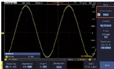
The Fine scale function is incorporated to allow users to fine tune the vertical scale according to their needs to achieve full scale measurement and improve the accuracy of the voltage or current measurements.
