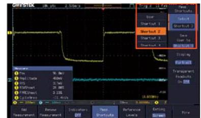
The GDS 3000A series soundly provides 38 measurement items. Based upon the parameters such as voltage, current, time, frequency, and delay measurement, users can decide which measurement items to choose. On the single display screen, the GDS 3000A series provides 8 measurement selections.
