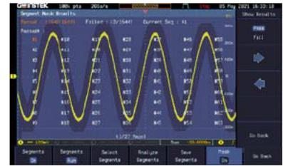
In addition, GDS-3000A incorporates the Mask determination function under Segment, allowing users to quickly analyze abnormal waveforms that exceed the target range.
