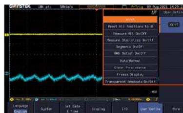
GDS 3000A incorporates a User Define key to allow users to set any one of the ten functions of User Define based upon the measurement requirement, including XY/YT; Reset all positions to 0; Measure all On/Off; Measure statistics On/Off; Segments On/Off; AWG output On/Off; Auto/Normal; Clear persistence; Freeze display and transparent readouts On/Off.
